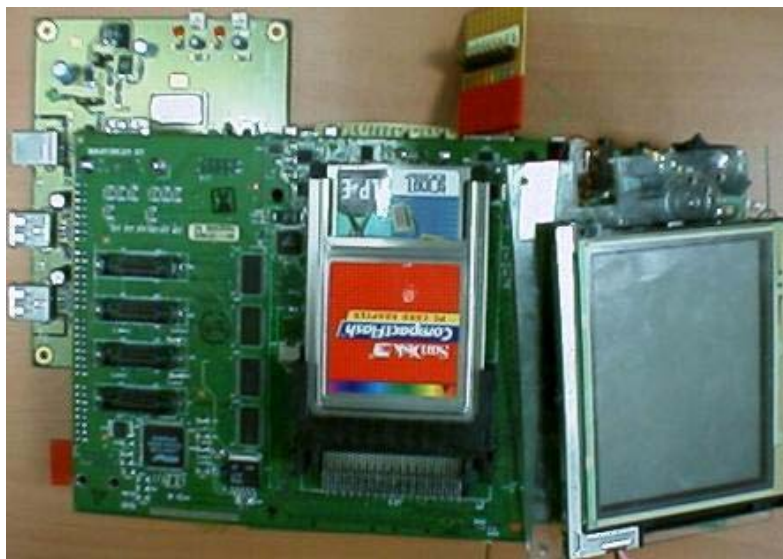
Figure A-4: ISPI161x Evaluation, StrongBridge, StrongARM Development Kit and StrongARM Companion Chip Development Kit
